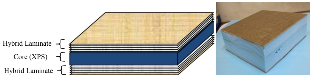
Fig. 1: Scheme diagram (left side) and picture (right side) of the developed hybrid composite panel
