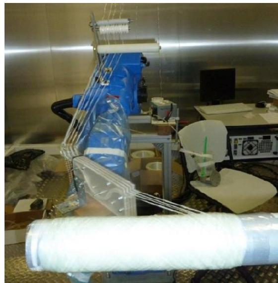
Figure 6. The filament winding with four roving.
