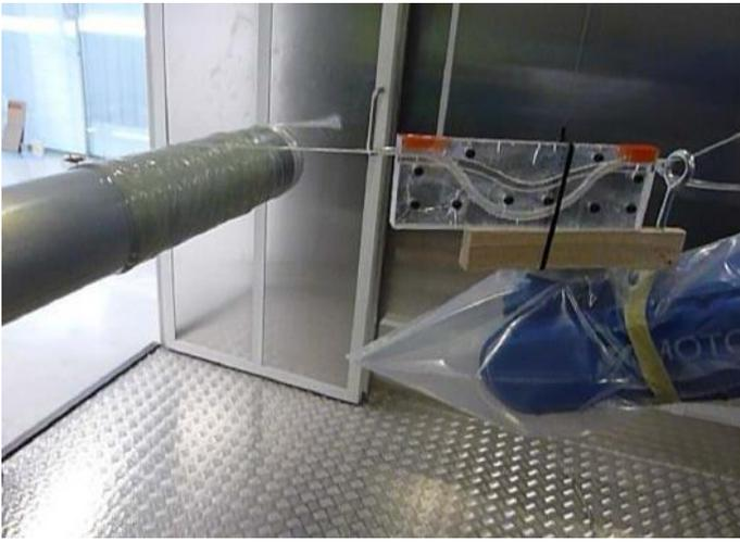
Figure 2. Syphon impregnation unit applied in the robot.
