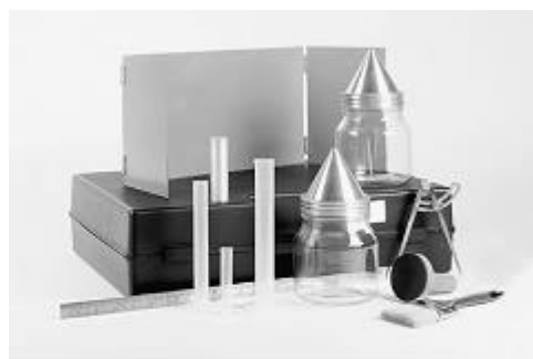
Fig. 7. Sand Patch apparatus (Model Controls).
