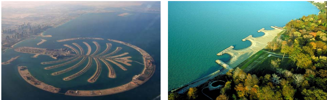
Figure 2.3: Examples of detached breakwaters.
