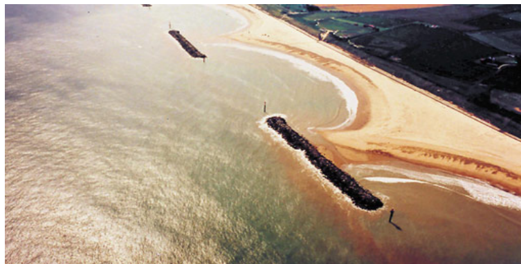
Figure 2.15: Formation of a tombolo in the leeward side of an emerged breakwater due to the diffraction currents.
