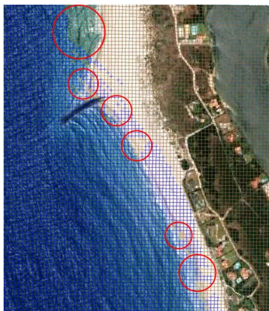
Figure 4.5: “Islands” created by the depth extrapolation (brown lines between blue lines).
