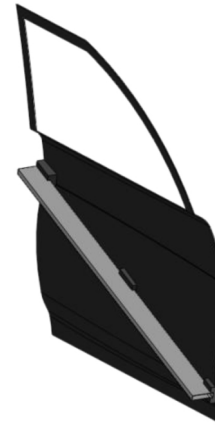
Figure 17. Optimized steel reinforced DCPD panel
