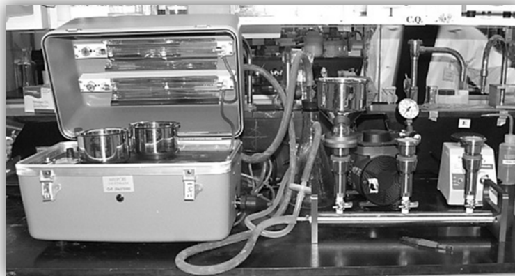
Figure 4.3 – Filtration system (Millipore Corporation, Billerica, MA): At the right, the 3-place standard manifold used for filtering the samples and, at the left, the UV box to sterilize the filter holders and funnels between filtrations [5].
