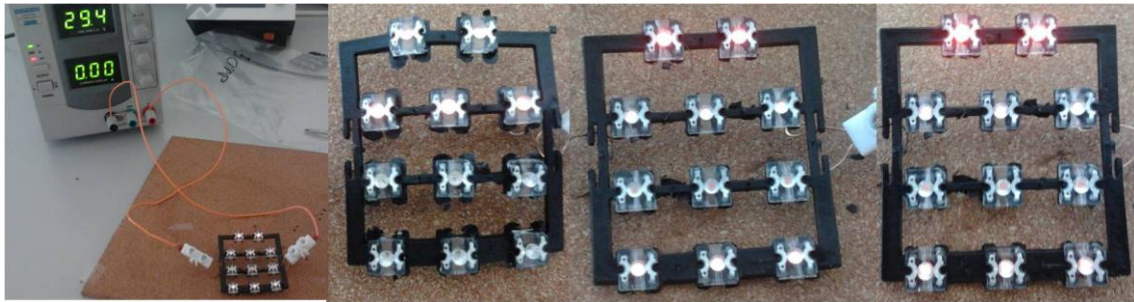
Figure 41 PP mixed with 5% (w/w) of CNT
