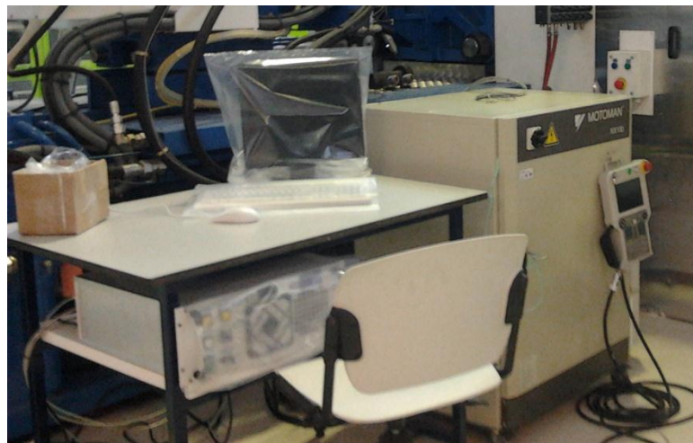
Figure 95 the laser and the NX100 robot control unit
