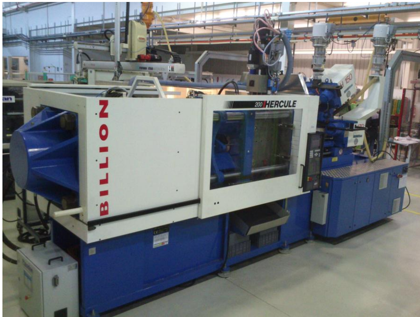
Figure 93 Billion with the vertical unit and the laser protection
