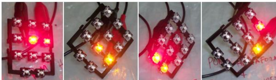
Figure 37 POM mixed with 4% of CNT
