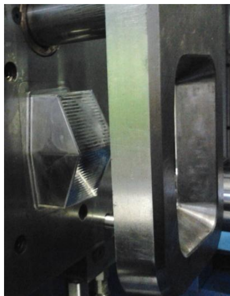
Figure 103 ejection and transport of the crystal component
