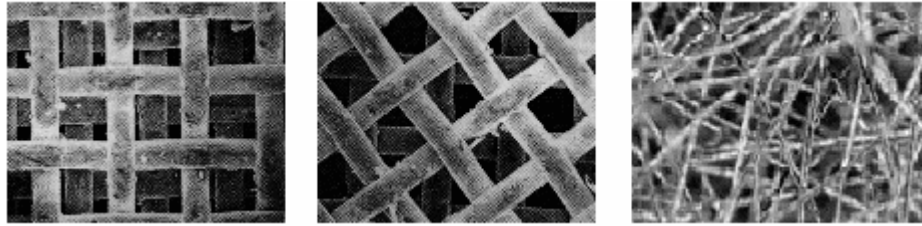
Figure 4.9 Microscope views of the matrix of three different regenerator matrices. Adapted from (Jiří, 2009).
