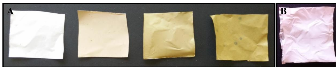
Figure 4.22 – Images showing the colour change of SELP-59-A fibres. (A) SELP/Ag fibres (from left to right) with 0, 1, 3 and 5 wt %; (B) SELP/LF fibres with 5 wt% bLF.
