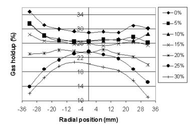
Figure 8 – Gas holdup radial profile for  $u_G$  = 0.046 m/s and solids loadings up to 30%v/v.
