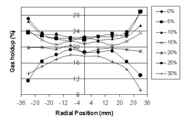
Figure 7 – Gas holdup radial profile for  $u_G = 0.038$  m/s and solids loadings up to 30% v/v.
