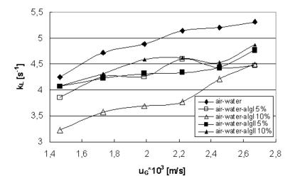
Figure 6 - Dependence of Liquid side mass transfer coefficient on superficial gas velocity, solids loading and solids size.
