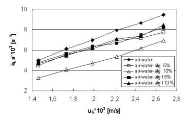
Figure 2 - Dependence of k<sub>1</sub> a on superficial gas velocity, solids loading and solids size.
