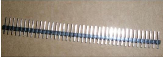
Figura 110 - Conector Arduino macho
