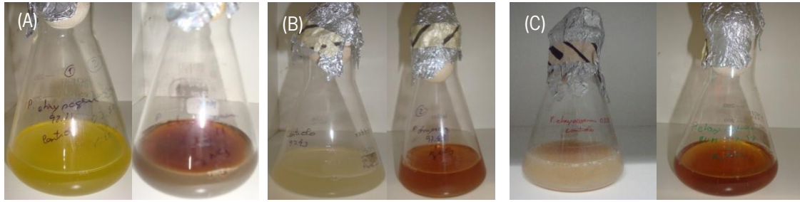
Figure 3 – Cellular filtrate of Penicillium chrysogenum MUM 97.43 (A), MUM 92.11 (B) and MUM 03.18 (C), treated with 1 mM of \text{AgNO}_3 after 96 h of incubation in the dark. Corresponding negative controls are shown on the left of each image.
