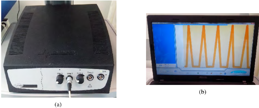
Figure 3.14: EMG Biofeedback System: (a) YSY EST EVOLUTION and (b) display with the device software.
