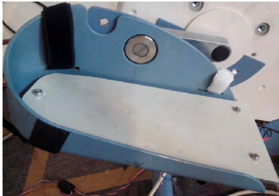
Figure 3.12: Right pedal with the mechanical system to measure the applied force.
