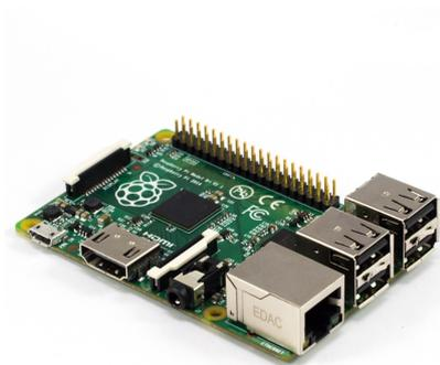
Figura 3.4: Raspberry Pi Model B+.
