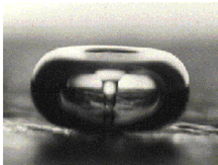
Fig. 6-12. Photograph of a collapsing cavitation bubble. Width of the bubble is approximately one mm. from University of Washington, Applied Physics Laboratory (Lawrence Crum, Ph.D.)
