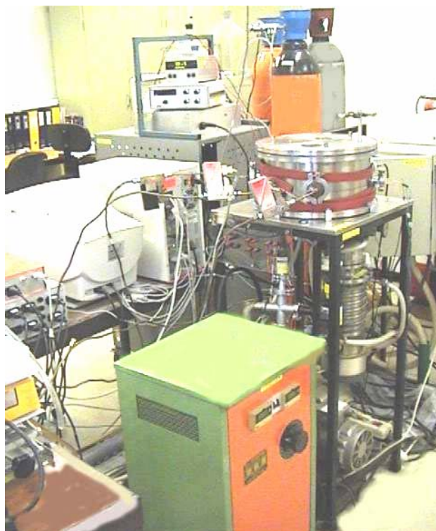
Fig. 2-3. Photograph of dc sputtering system.
