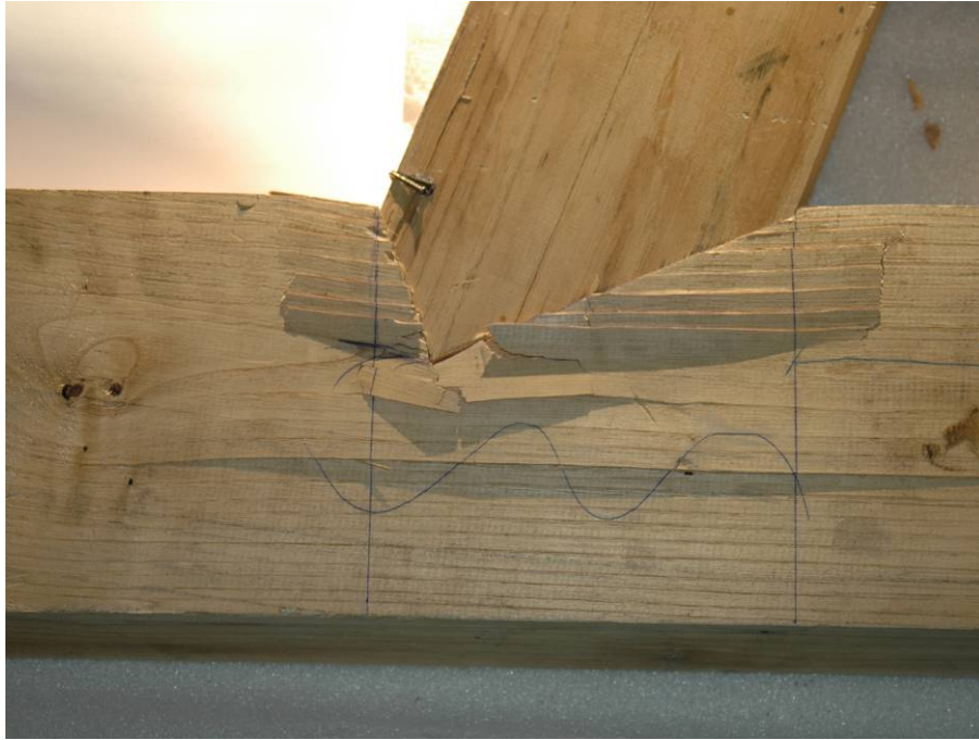
Figure 4 – Typical experimental failure patterns observed: (a) joint collapsed in compression, with uniform distribution of damage, (b) joint collapsed in compression, with out-of-plane bulging, and (c) combined failure in compression and shear parallel to the grain at the toe.
