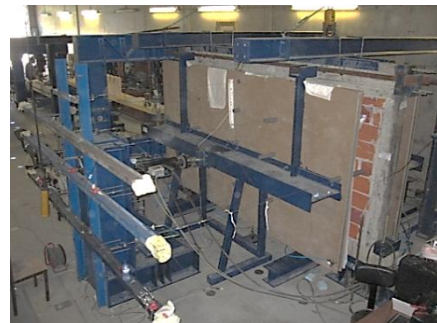
Label: 1 – Reaction frame; 2 – Upper support beam; 3 & 4 – Airbags Structure; 5 – Airbags support; 6 – Horizontal hydraulic jack.
