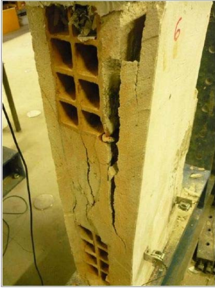
FIGURE 5 Failure mode of the masonry prisms tested.
