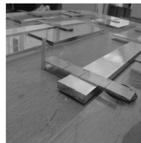
c) Detail of the spacer and adhesive bond
