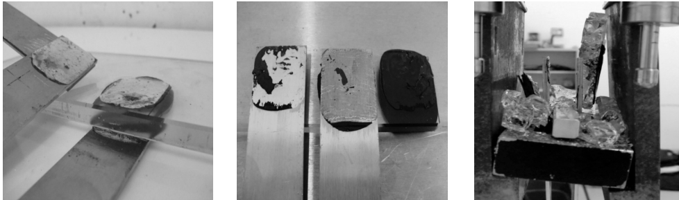
Figure 5: Failure modes for the monotonic tests: Adhesive failure (left); failure at the steel/adhesive interface (center); glass failure (right)
