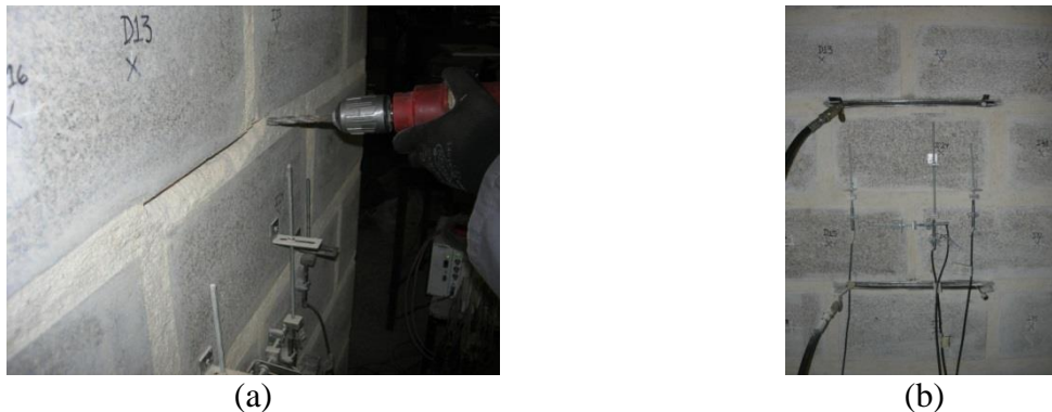
Figure 11 Double flat-jack test set-up: (a) drilling the second slot; and (b) the complete set-up
