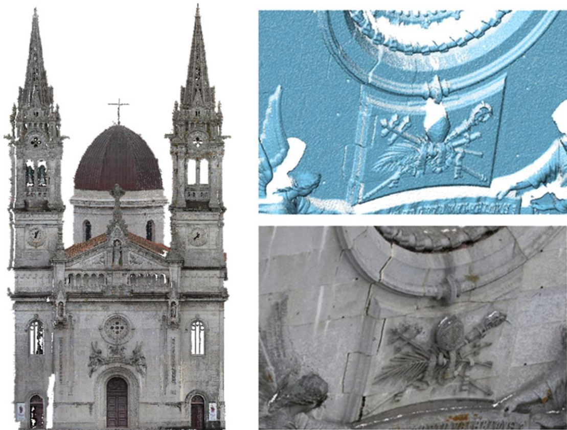
Fig. 7. Front elevation of the point cloud obtained through SfM technique and PW software (Left). Detailed comparison between the laser scanner point cloud and the one obtained in PW software (Right).
