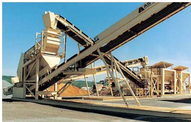
Figure 6 – Classification system for incorporation of recycled material in continuous plant (adapted from Fonseca (2005))
