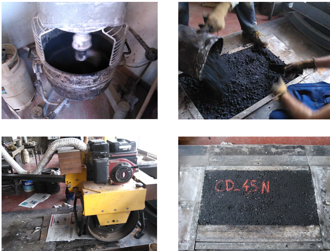
Figure 32 – Procedures use to produce an asphalt mixture and to compact a slab
