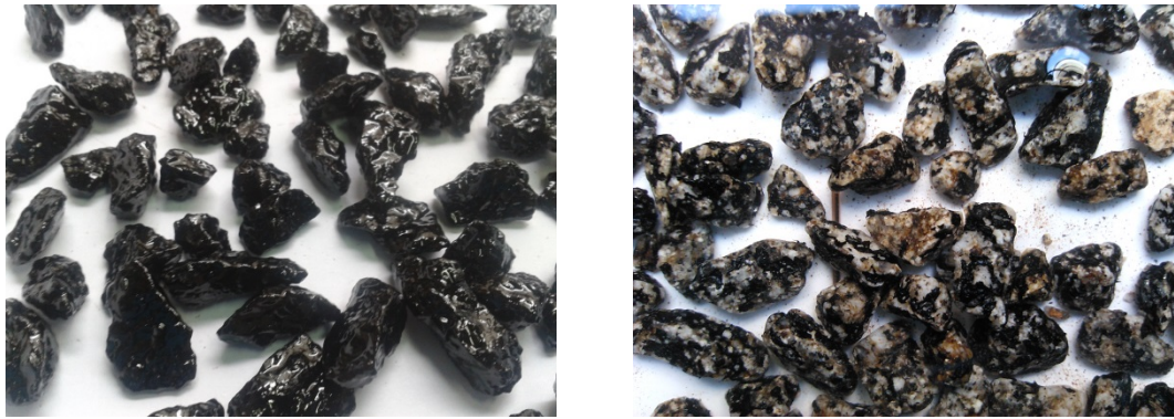
Figure 47 – Surface of the aggregates covered by bitumen before and after the affinity test
