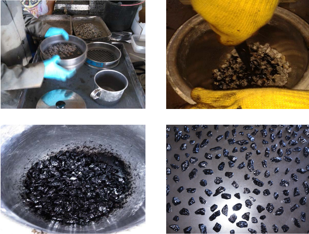
Figure 26 – Preparation of the aggregates covered with bitumen for the affinity test
