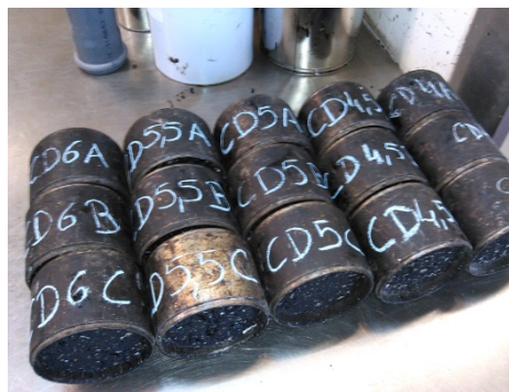
Figure 23 – Five groups of specimens used in the Marshall test to determine the optimum binder content
