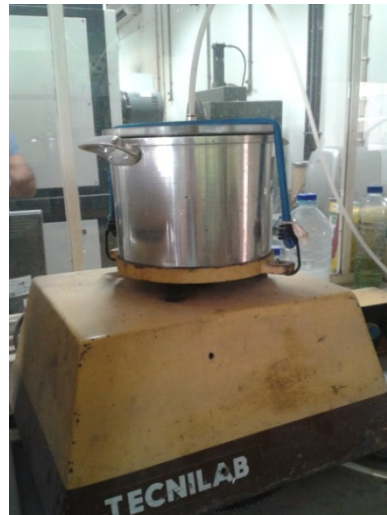
Figure 25 – Pycnometer used in the determination of the maximum theoretical density
