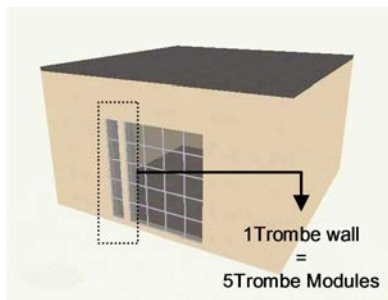
Figure 3 Model: One Trombe wall.
