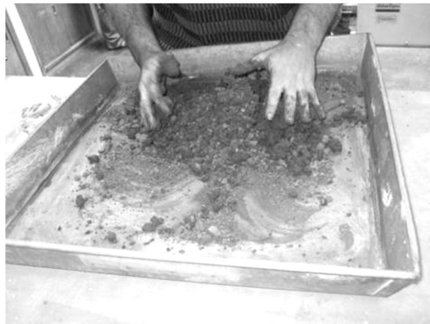
Figure 5.19 – Mixing of the soil with water: clay sticking to the hands and formation of agglomerates.
