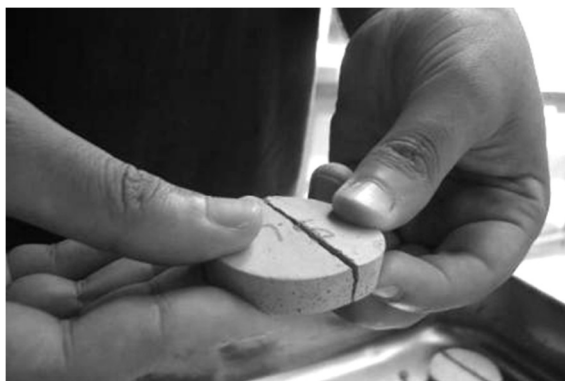
Figure 5.6 – Execution of the dry strength test.
