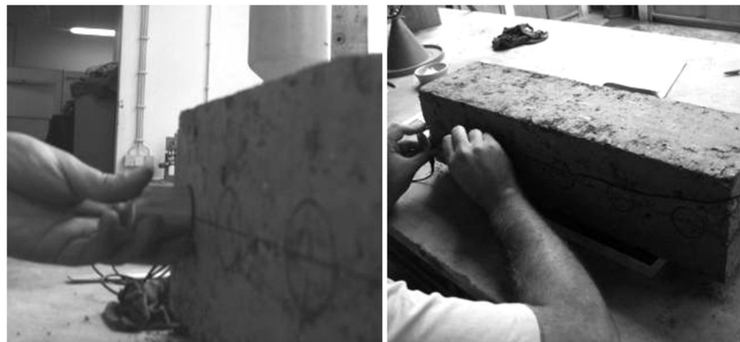
Figure 6.19 – UPV measurements on the medium-scale specimens.
