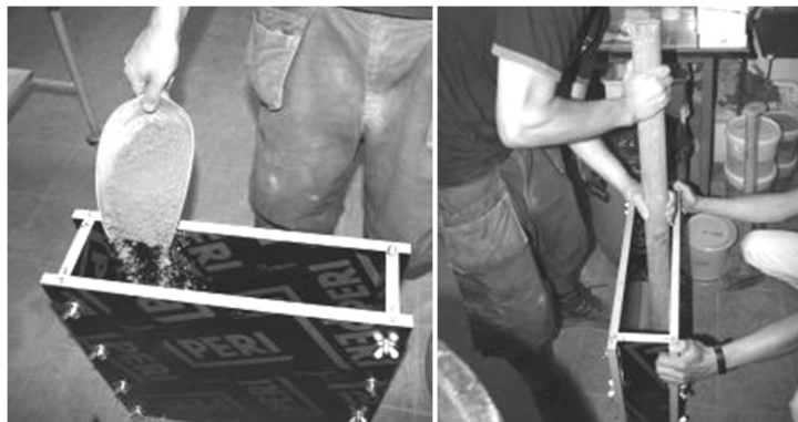
Figure 7.1 – Manufacture of the rammed earth wallets tested by BAM-ZRS.
