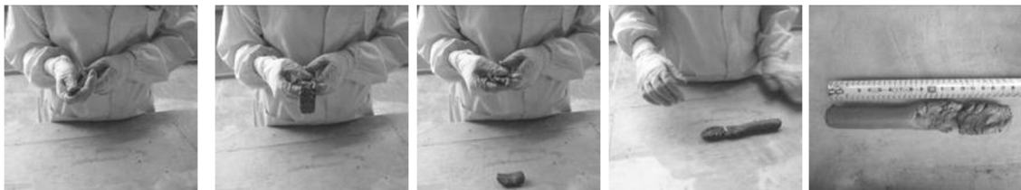
Figure 5.4 – Sequential execution of the ribbon test.
