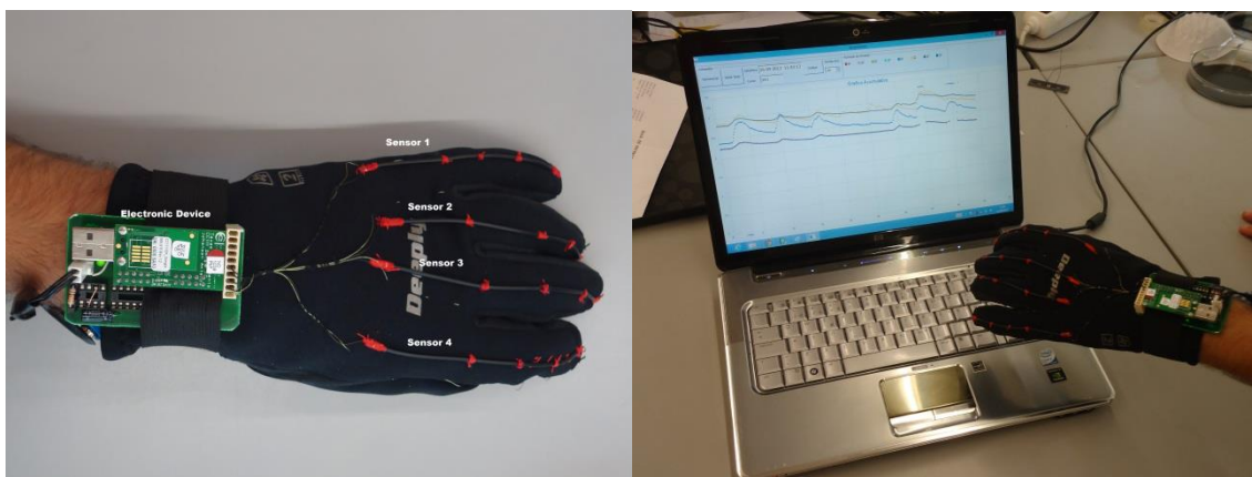
Figure 7.3- Images of the glove with the extruded composite C540 CNT/SBS with 8 wt% CNT filler content for measuring finger deformation via wireless data transmission.
