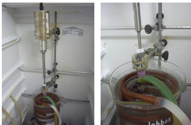
Figure III.1. Pictures of the Ultrasonic equipment used along this work for silk fibroin nanoparticles production. The samples placed in ultrasonic flasks were putted in contact with an ultrasound probe.
