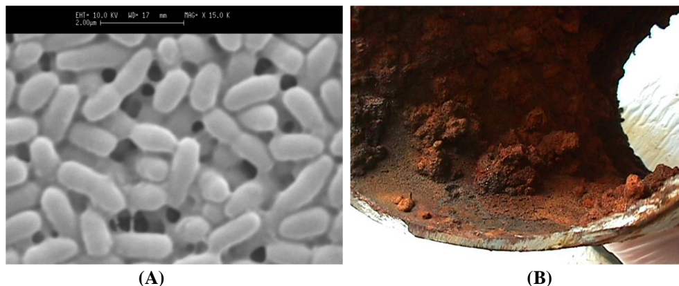
Figure 1. (a) Scanning electron microscopy (SEM) photomicrographs of 24 hours old biofilms formed by the opportunistic Gram-negative Burkholderia cepacia (isolated from laboratorial DWDS) evidencing the presence of an extracellular polymeric matrix ( \times 15000 magnification; bar = 2 \mu\text{m} ). (b) Ductile iron pipe section from a DWDS with biofilm and high amounts of corrosion products. This section of DWDS was obtained as result of a pipe break in the DWDS.
