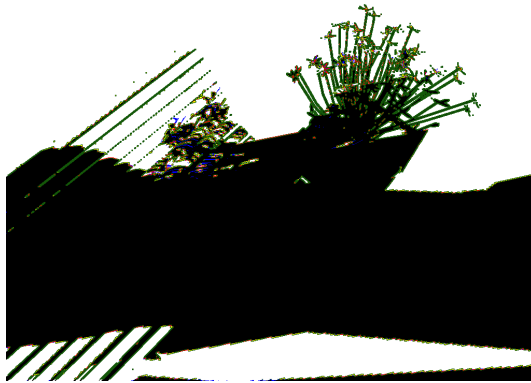
Figure 50: Worst case of shadow map errors being caught inside contours with a 2048x2048 shadow map.
