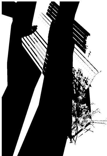
Figure 66: Worst case of only information of nine neighbouring texels with a 2048x2048 shadow map.
