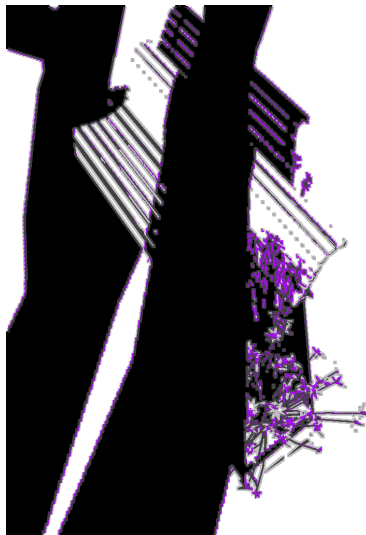
Figure 230: Result of the algorithm with a six pixel thick contour and a 2048x2048 resolution shadow map for the with viewpoint of the flowers scene.
