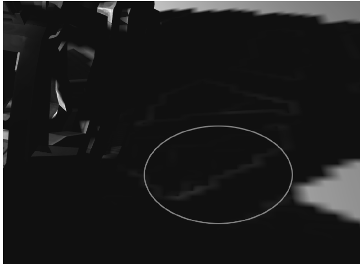
Figure 8: Variance Shadow Map light leaking example.
