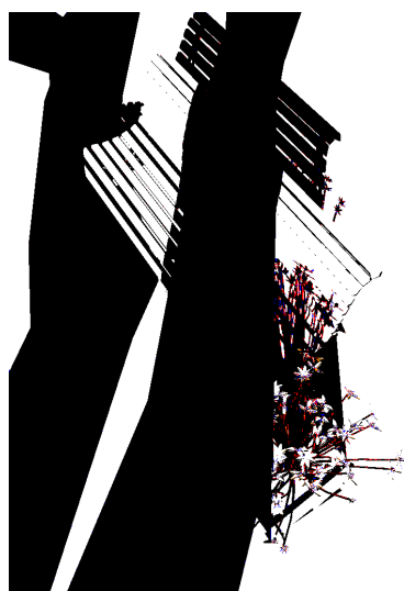
Figure 87: Marked errors of the worst case when using a 2048x2048 shadow map.
