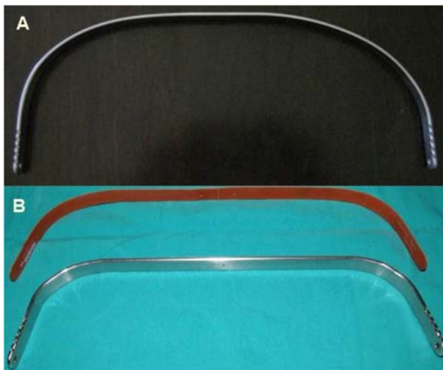
Fig. 5. Representation of the differences between two bended prosthesis: (A) bended manually and (B) bended using the i3DExcavatum system.
