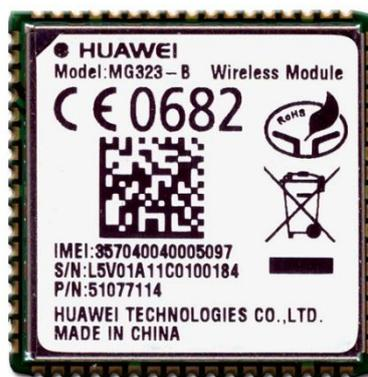
**Figura 29: Huawei MG323 [21].**
