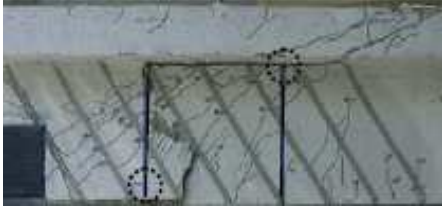
Figure 10: Crack patterns of the beams (in pink colour: crack completely open; in red colour: crack in the opening process; in cyan colour: crack in the reopening process; in green colour: crack in the closing process; in blue colour: closed crack).
