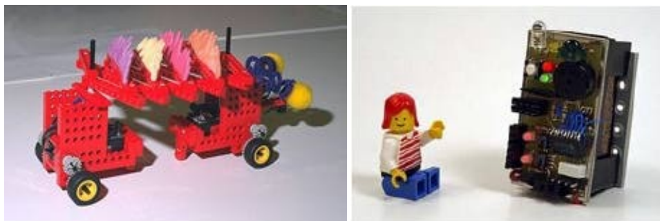
FIGURE 3-6 Robotic construction with two built-in Crickets, which communicate with one another to synchronize their motion, reproduced from (Resnick et al. 1998).
