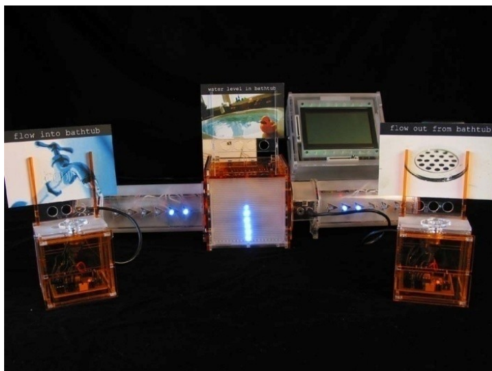
FIGURE 3-9 System Blocks simulating water flow through a bathtub, reproduced from (Zuckerman 2004).
