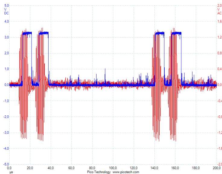
Figure 6.12: Result of OOK demodulation with PVDF transducer.
