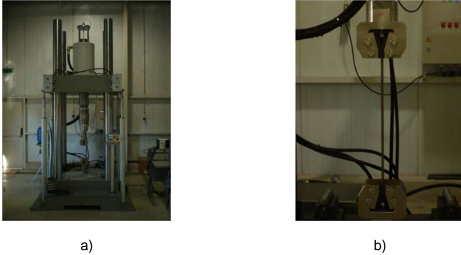
Figure 5.17. Laboratory tests: a) uniaxial tension test; b) reinforcing steel specimen.
