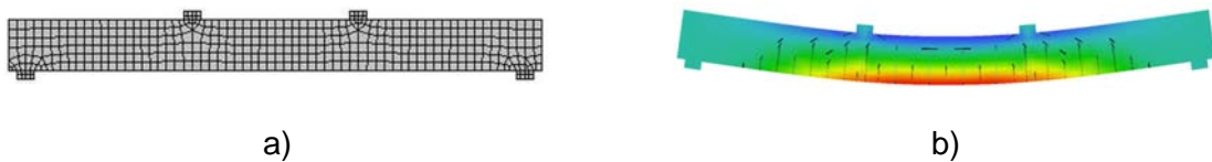
Figure 5.8. Numerical model: a) finite element mesh; b) failure mechanism.
