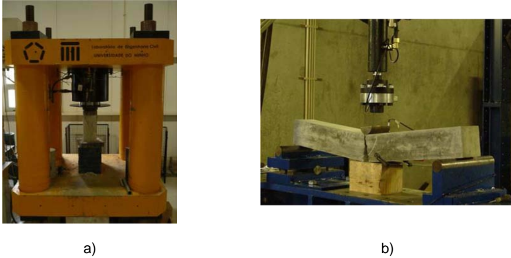
Figure 5.16. Laboratory tests: a) uniaxial compression test; b) fracture energy test.
