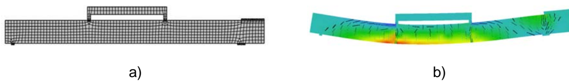
Figure 5.9. Numerical model: a) finite element mesh; b) failure mechanism.
