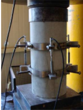
Figure 2: Test setup for Modulus of Elasticity
