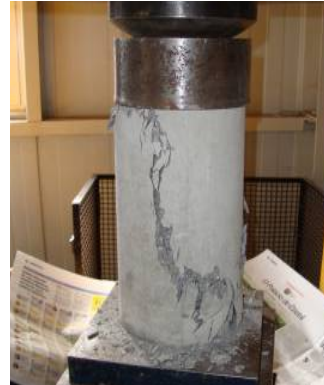
Figure 3: Test setup for stress-strain in compression
