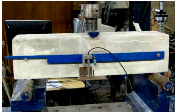
Figure 5: Test setup for the bending test
