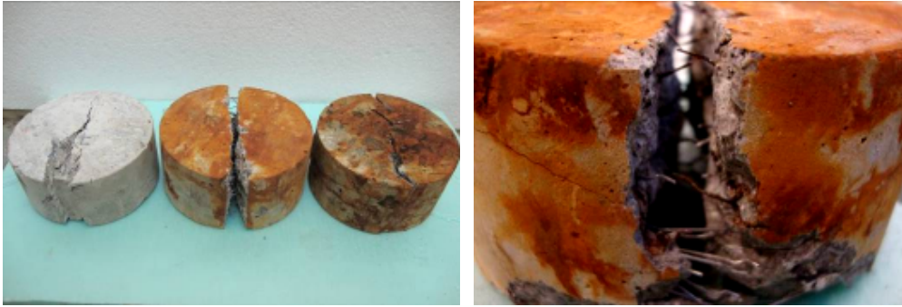
Figures 14: SFRSCC specimens after and before chloride migration test (left) and after tensile test by diametral compression (right)
