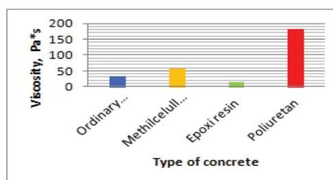
Fig. 1. Apparent viscosity of the compositions studied
