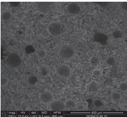
Fig. 7. Methylcellulose concrete at 28 days after casting
