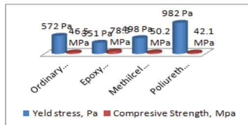
Fig. 4. Correlation between compressive strength and yield stress
