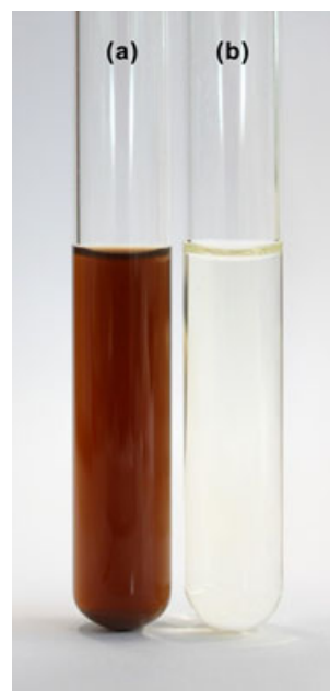
Figure 3. Olive oil mill wastewater pictures at the beginning (a) and at the end (b) of the photocatalytic treatment.
