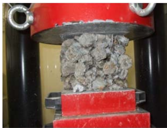
b) Corn cob concrete sample
