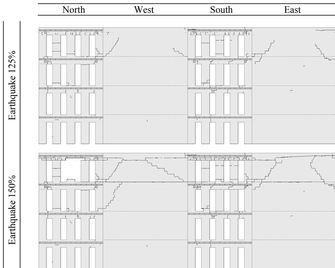
Figure 3.6 – Crack patterns of the strengthened mock-up: Earthquake 125% and 150%.
