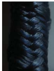
Fig. 2– Surface of braided structure
