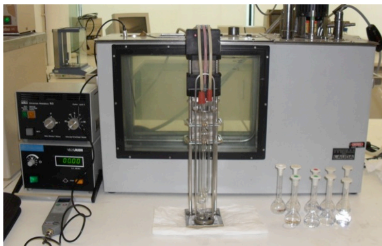
Figure 3.5 – Representation of the equipment used to measure the intrinsic viscosity.
