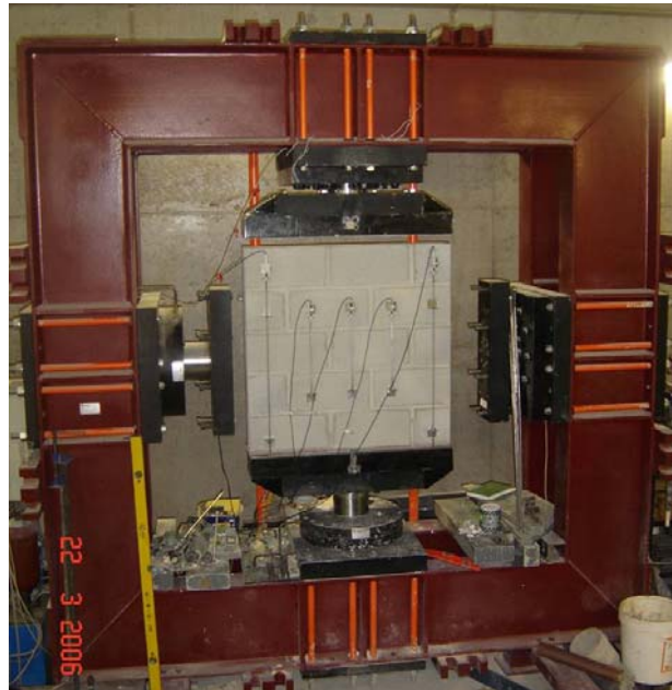
Figure 4: Overall view of hydraulic servo-controlled machine test.
