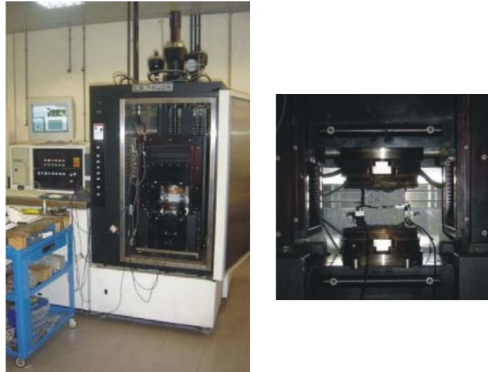
Figure 2: Tensile test machine and the concrete sample.
