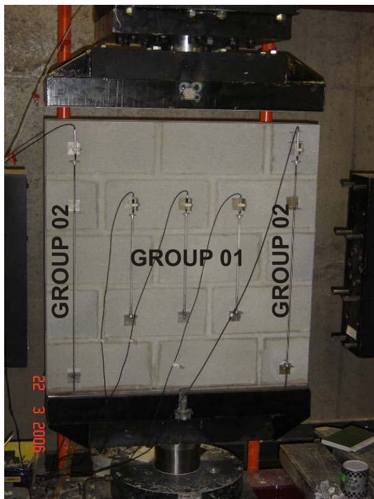
Figure 5: Positioning of LVDTs groups for compression tests of masonry.
