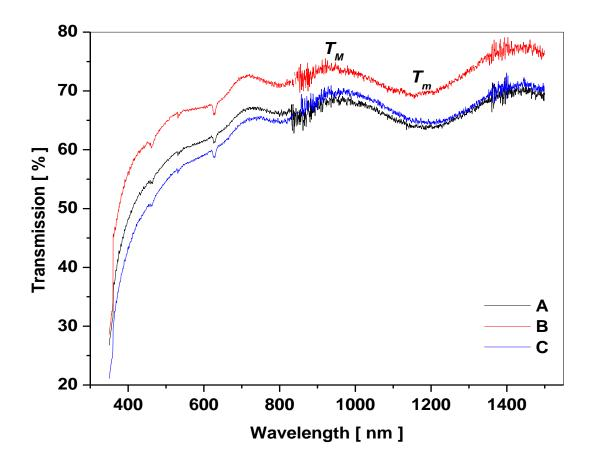
Fig.3. Transmission spectra of  $TiO_2$  thin films deposited on FTO glass substrates.
