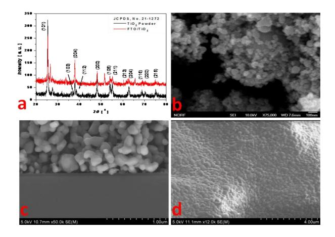
Fig.1. (a) XRD patterns of TiO<sub>2</sub> nanoparticles, TiO<sub>2</sub> coated on FTO glass, HR-SEM images of (b) TiO<sub>2</sub> nanoparticles, (c) Cross-section view and (d) plane view of TiO<sub>2</sub> coated on FTO glass.
