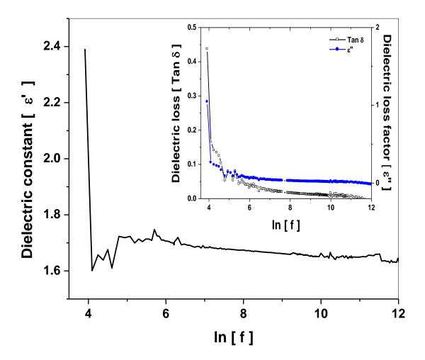
Fig.2. Variation of dielectric constant ( $\varepsilon'$ ) of FTO/ TiO<sub>2</sub> and the inset shows the variation of dielectric loss ( $tan \delta$ ) and dielectric loss factor ( $\varepsilon''$ ) of FTO/ TiO<sub>2</sub>
