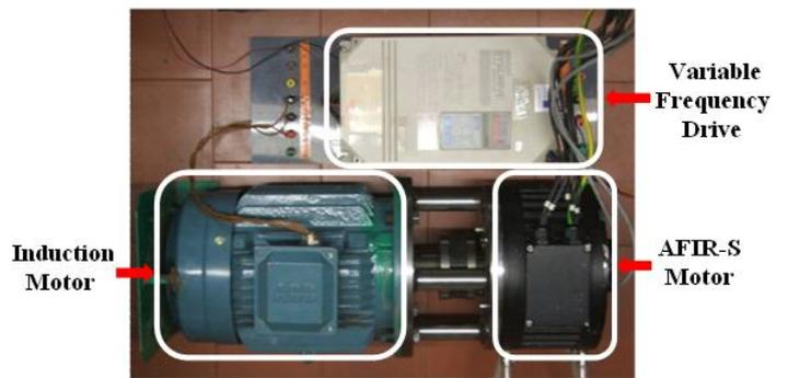
Fig. 7. Test bench assembled to synchronize the AFIR-S windings.
