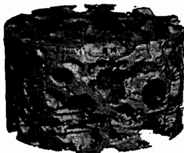
3 Three-dimensional microcomputerised tomography ( \mu CT) image of scaffold obtained by extrusion of SEVA-C (blend of starch with ethylene vinyl alcohol) with blowing agent
