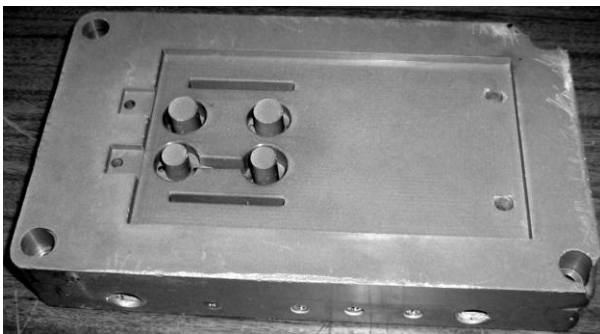
Figure 6 – Composite moulding block after successive injection cycles.
