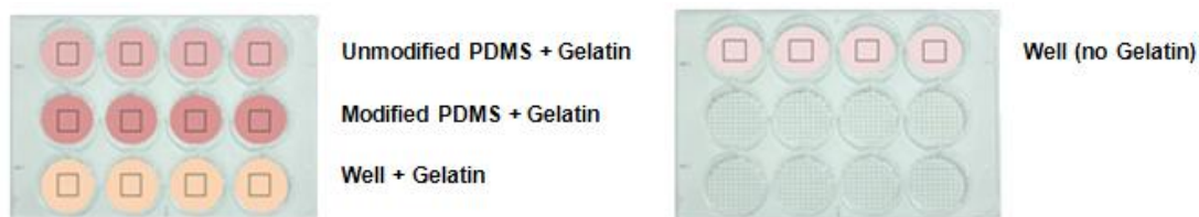
Figure 15. Distribution of PDMS samples in the 12 well-plate, for the second experiment with HUVECs. In the left plate, the first 4 wells contain unmodified PDMS surfaces with adsorbed fibronectin, the next 4 contain modified PDMS surfaces with adsorbed fibronectin and the last 4 wells only contain a fibronectin coating. In the second plate, the first 4 wells have no additional surface or coating. Both the 12 well-plate were prepared in triplicate, one to be incubated for 3 days, the other for 4 days and the last for 5 days.
