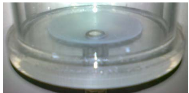
Fig 3: Filtration column detail: bottom retention structure
