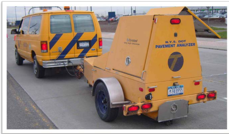
Figura 3-18 - Falling Weight Deflectometer (FWD)
